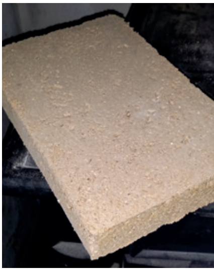
One of the pre-production insulation panels tested, 62mm (2½") thick
